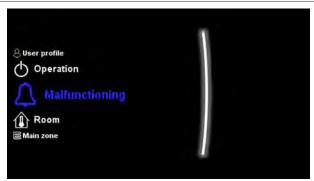
Press? in the error screen. **Result:** A long description of the error is displayed on the screen.
