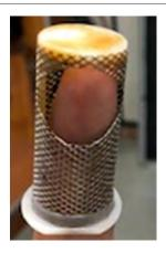
**5** When cleaned, reinstall the filter in the shut-off valve.
