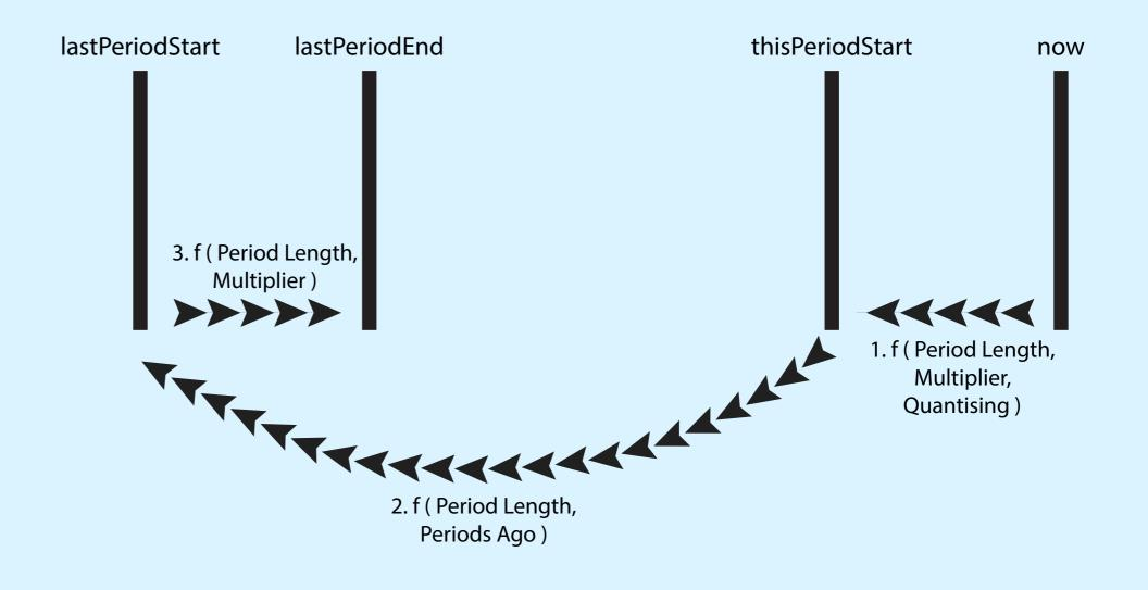
The 'time window' is the calculation period, for example between 'now' and 'thisPeriodStart'. The arrows indicate the calculation procedure, and the variables included in the calculation function f(x).
