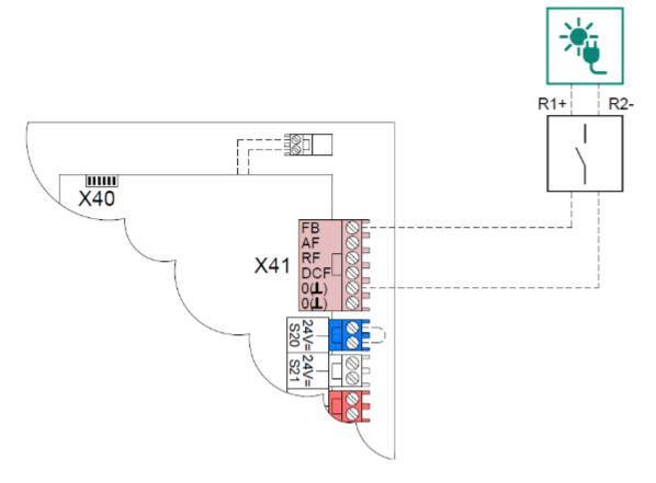
The "FB and OT" contact of socket X41 on the printed circuit board
