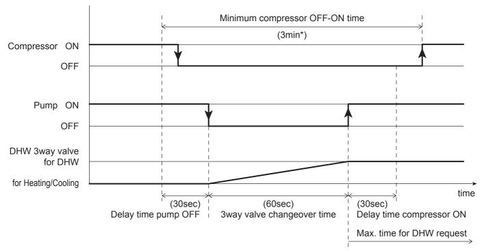
\*Minimum compressor OFF-ON time (3min) is a fixed value. The interval time is necessary for refrigerant cycle safety, it cannot be changed.
