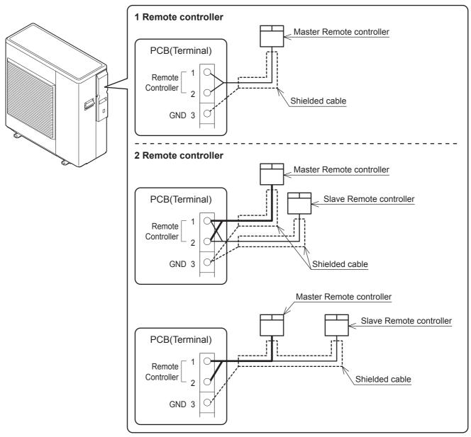
• The maximum length of the Remote controller cord is 100m. Use shielded wire in case of the length with 30m or longer. Connect the shielded wire to Terminal No.3(GND) on the PCB(Terminal).
