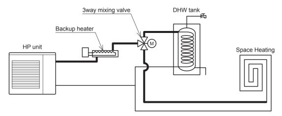
A parameter defines if the Backup heater can be enabled or disabled, and the "Type of function": Heater in Replacement mode
