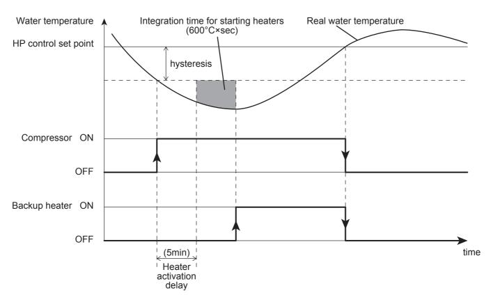
The "HP unit control set point" is equal to the value set for Fixed set point control, or by the value determined by the Climatic curve.
