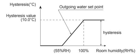
Note: If the HP unit is connected directly to the system, without Buffer tank, the maximum Room humidity compensation has effect on the Outgoing water temperature from the HP unit. If the HP unit is connected to the Buffer tank and the low temperature Zone with a 3way mixing valve is enabled, the maximum Room humidity compensation has effect on the Outgoing water temperature from mixing valve.
