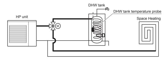
The DHW can be heated as following configuration by setting Par3102.
