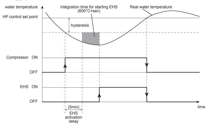
The "HP control set point" is equal to the value set for Fixed set point control, or by the value determined by the Climatic curve.
