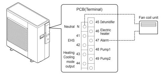
In case of Par0400=1, if the Room air temperature detected by the Remote controller has not reached the set point, the Terminal47 will be closed.
