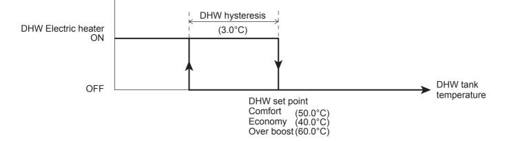
If the Par3102=2 (Heater only), the heat pump produces hot or cool water for the system and the hot water will be heated by the electrical heater only.
