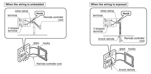
• Do not damage the PCB of Remote controller with too much pressure when the terminal is installed.
