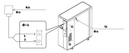
The maximum length of probe cables is 100m for 1mm<sup>2</sup> cables, and 30m for 0.5mm<sup>2</sup> cables.
