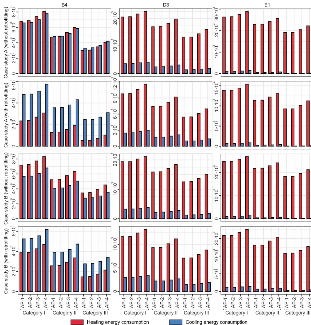
Fig. 9. Distribution of the annual energy consumption obtained in the case studies with the approaches of adaptive setpoint temperatures in 2050.
