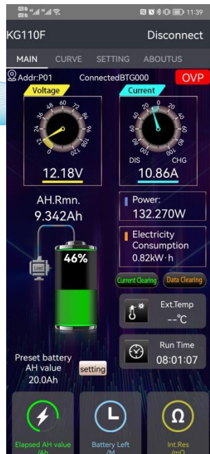
Figure 3-5-12 Over-voltage protection status
