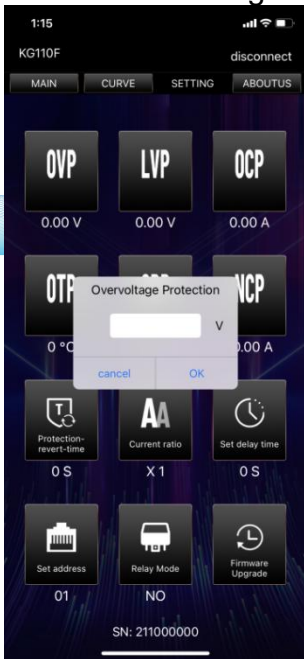
Figure 3-5-67 Input Over-voltage Protection
