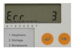
Regardless in which menu you are in the Supercal 531: after 3 minutes the integrator returns automatically to the first display of the main menu.
