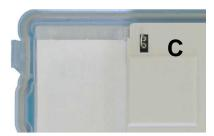
The jumper for the calibration mode has to be plugged in here. The calibration-relevant functions can only be activated and set over the optical interface with the service software Prog531.
