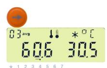
Alternatively, the display sequence for the requested average value can be selected by pressing the enter key.
