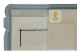
When replacing the battery, the calibration seal is damaged! Therefore, only personnel authorized and trained by Sontex may carry out the replacement. In case of improper handling, the warranty of Sontex is void!
