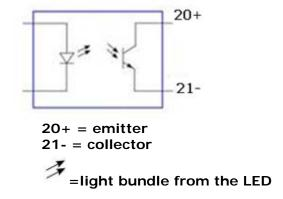
The pulse output is 1000 per kWh and is settable using the RS485 communication protocol, the table below outlines the possibilities.
